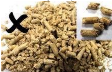
Poor quality pellets
