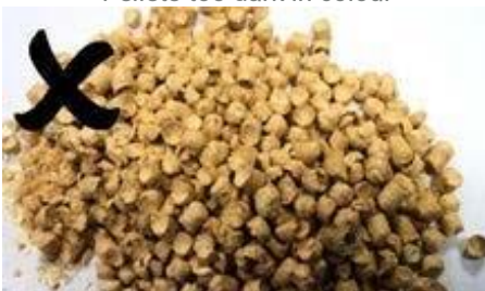
Pellets too short in length
