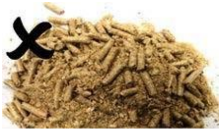
Pellets with high dust content
